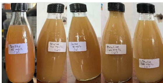
Figure 4. Synthesis Results of Dexlite-Nano TiO 2 with loading of 40, 80, 120, 160 and 200 mg/L.
