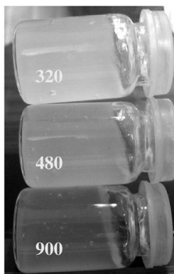
Figure 4. CNF Gel Produced by the Method of Delignification Followed TEMPO-Mediated Oxidation Pretreatment, and Blending Using High Speed Blender (Boufi and Chaker, 2015).
